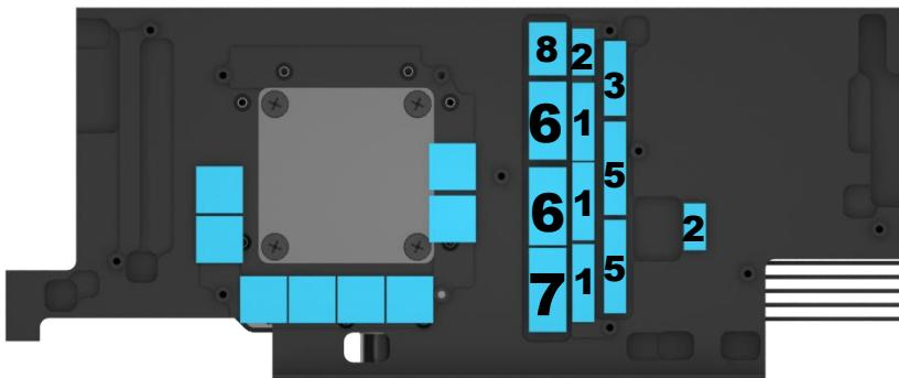
**EN** Remove the protective film from the cooler base and clean the contact surfaces on the base side of the cooler with spirit or similar agents. The surface must be free of contaminants.
