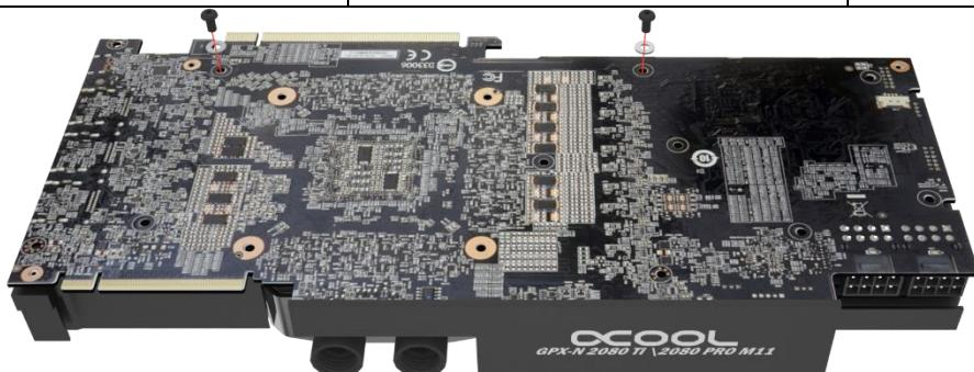
**EN** Place the graphics card on the cooler as shown in the picture. Mount the graphics card with 2 M3x6 screws and M3 washers as shown in the picture.
