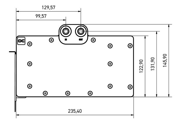
General tolerance: ± 0,25mm Dimension in millimeter
