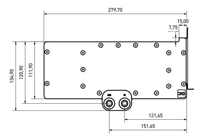
General tolerance: ± 0,25mm Dimension in millimeter
