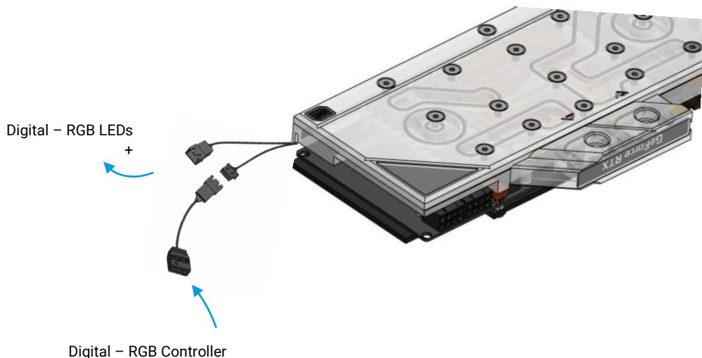
**EN** To control the digital - RGB lighting, connect the included adapter to the 3 - pin female connector and plug it to a digital - RGB controller (e.g. Alphacool Aurora Eiscontrol, Art.: 15360, not included). You can connect additional digital - RGB LEDs to the remaining 3 - pin male connector.
