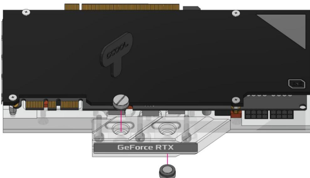
**EN** Close the inlets which you do not need for tubing. Screw in the screw plugs with the enclosed tool.
