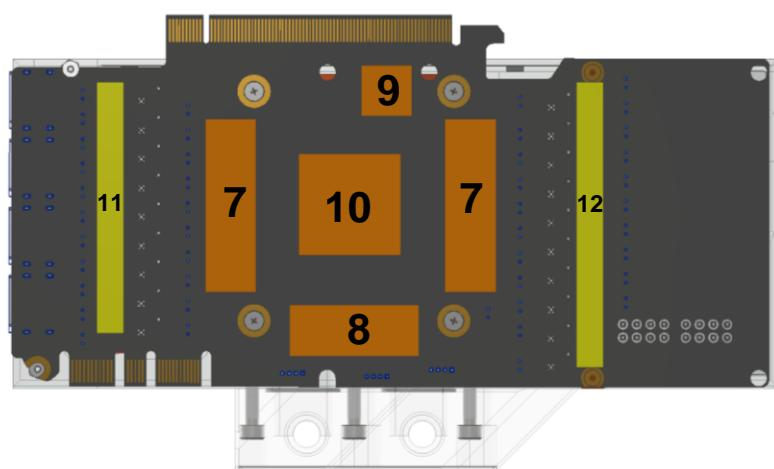
**EN** Remove the protective foils from the thermal pads and place the pads on the PCB as shown.
