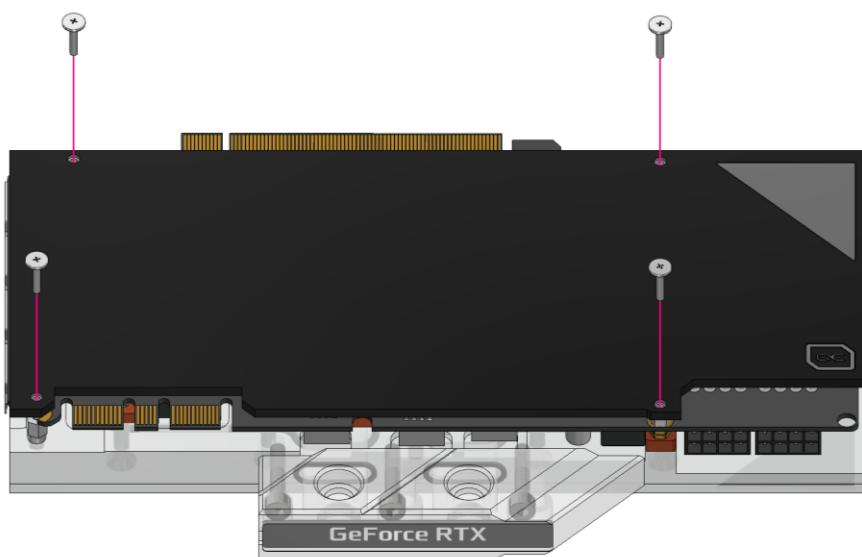
**EN** Put the backplate on and screw it together with the 4 M2x11 screws as shown.
